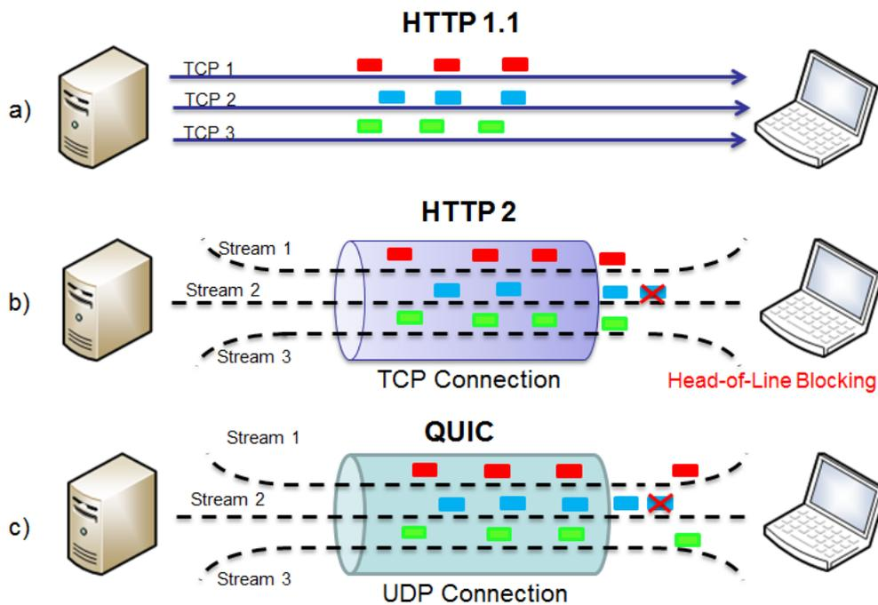
Figure 2. Multiplexing Comparison
