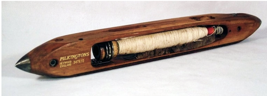
Fig. 3.7: A typical flying shuttle, invented by John Kay in 1733. The shuttle contains a spool, onto which the weft yarn is wound.
