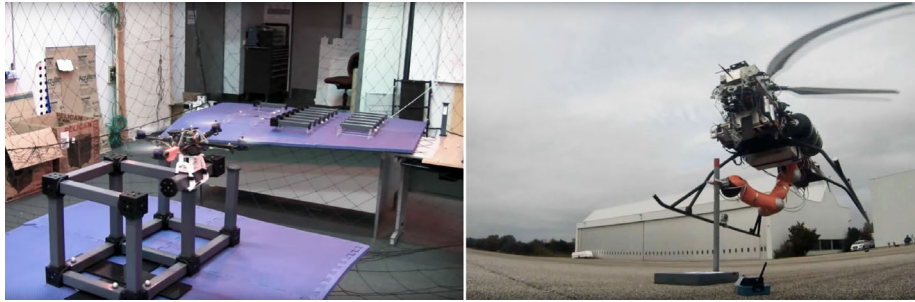
Fig. 2.11: On the left, construction of cubic structures using bars with magnetic joints (GRASP Lab, University of Pennsylvania, 2011) [55]. On the right, assembly of a space truss structure using a robotic arm mounted on a robotic helicopter (DLR, 2013) [58].
