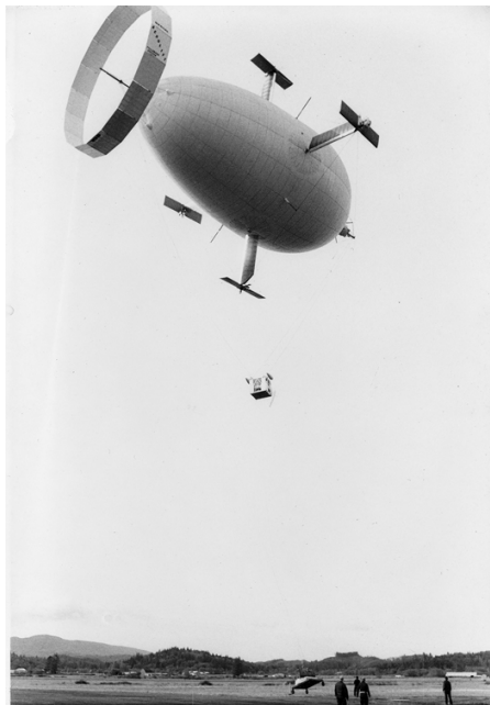
Fig. B.5: On the left, the CycloCrane during its first manned flight in Tillamook, OR, in 1984 [191]. On the right, a drawing from the CycloCrane patent, indicating the principle [192]. The person operating the vehicle sits in a cabin between the payload and the machine, suspended from the airship.
