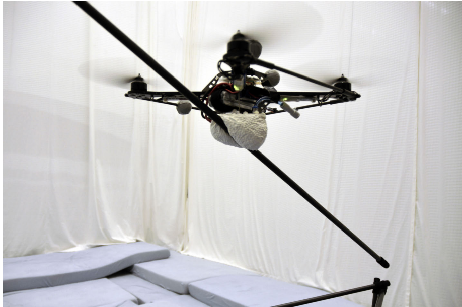
Fig. C.2: Jamming gripper. The gripper uses negative pressure to compress granular filling material (Styrofoam balls) contained in a membrane (balloon) to rigidly grasp a round carbon tube at variable angles.
