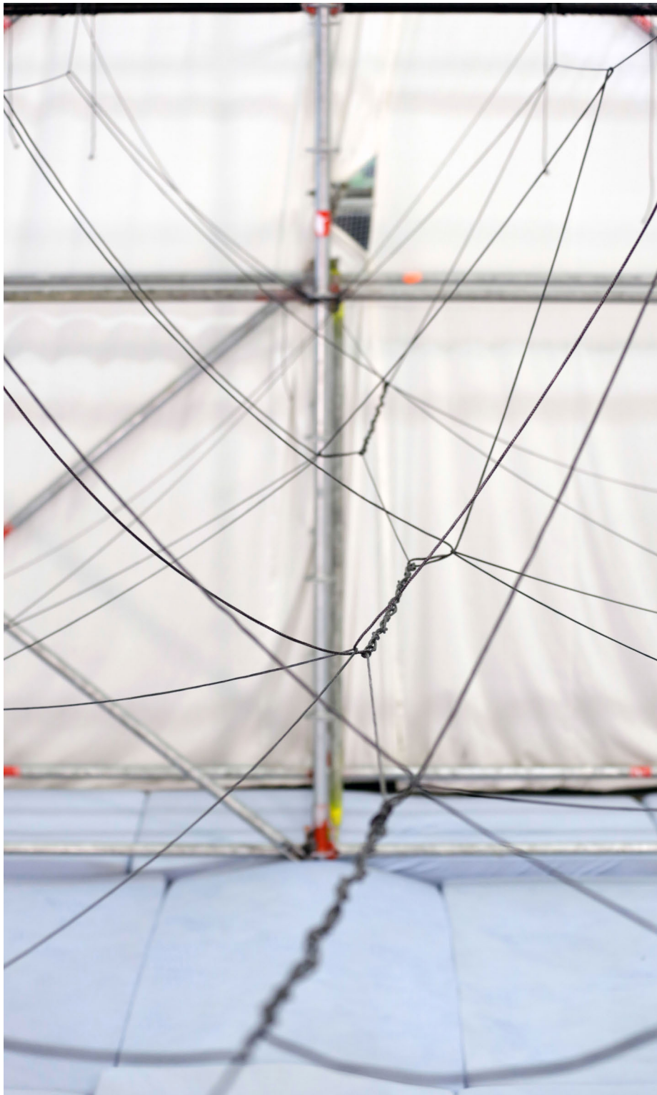
Fig. 5.27: Detail view of the final structure. The stabilising elements distorted the braid segments due to their non-symmetrical arrangement.
