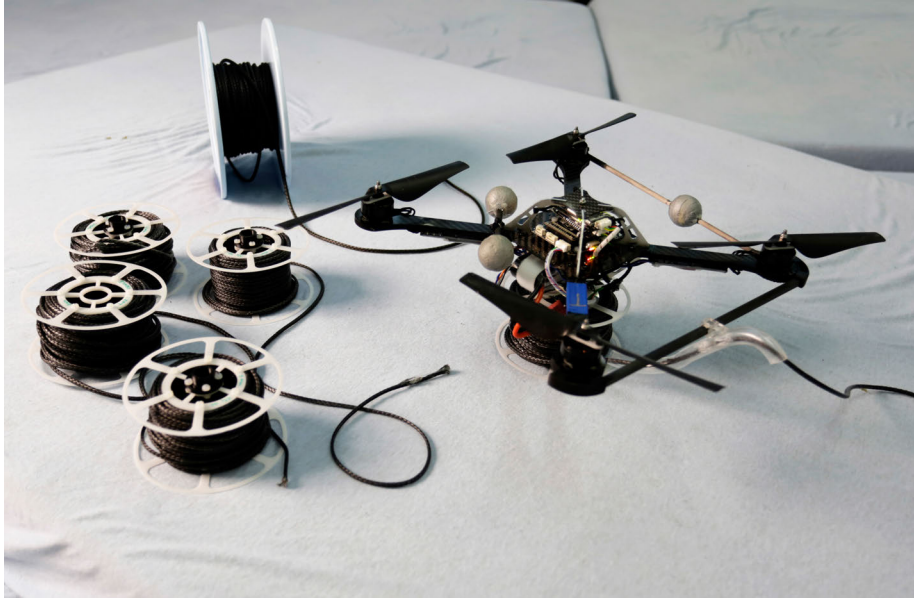
Fig. 5.1: Quadcopter and wound spools with different lengths of 4 mm Dyneema rope.
