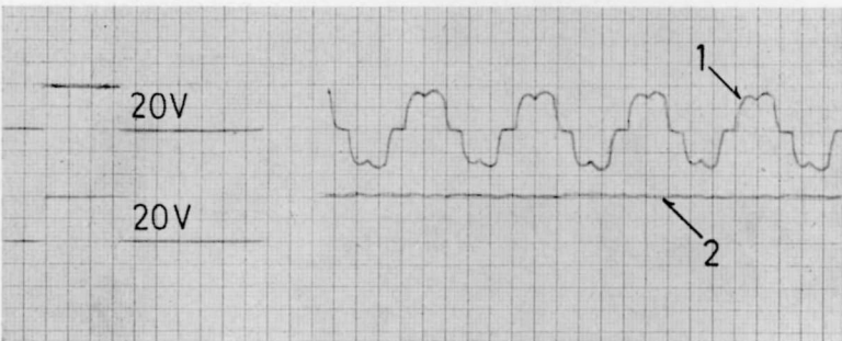
Fig. 34e Phase current i_1^r and the field current i_f^r 1 = 0.25 L_d^r i_1^r 2 = 0.2 i_f^r
