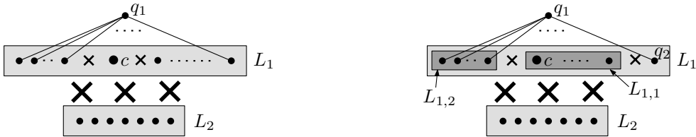
Figure 4: Construction of a graph G for which any algorithm needs \sqrt{n} queries to discover a maximal independent set
