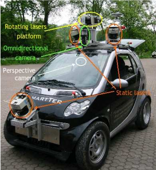
Figure 6.1: Our experimental robotic platform SMARTER with which we participated in ELROB (the first European Land Robot Trial) [97].
