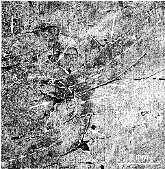
Figure 5.11: Tension surface (bottom) of a CF/PEEK sample subjected to low energy impact. The cracks were initiated along the bundle/matrix interface (arrows) and therefore, reflect the knitted CF bundle structure (A). This observation confirms the crucial role of bundle/matrix interfaces in knitted CF reinforced PEEK. Bundles released from their environment were the smallest units in all observed fracture zones (see also fig. 5.5, chapter 4).
