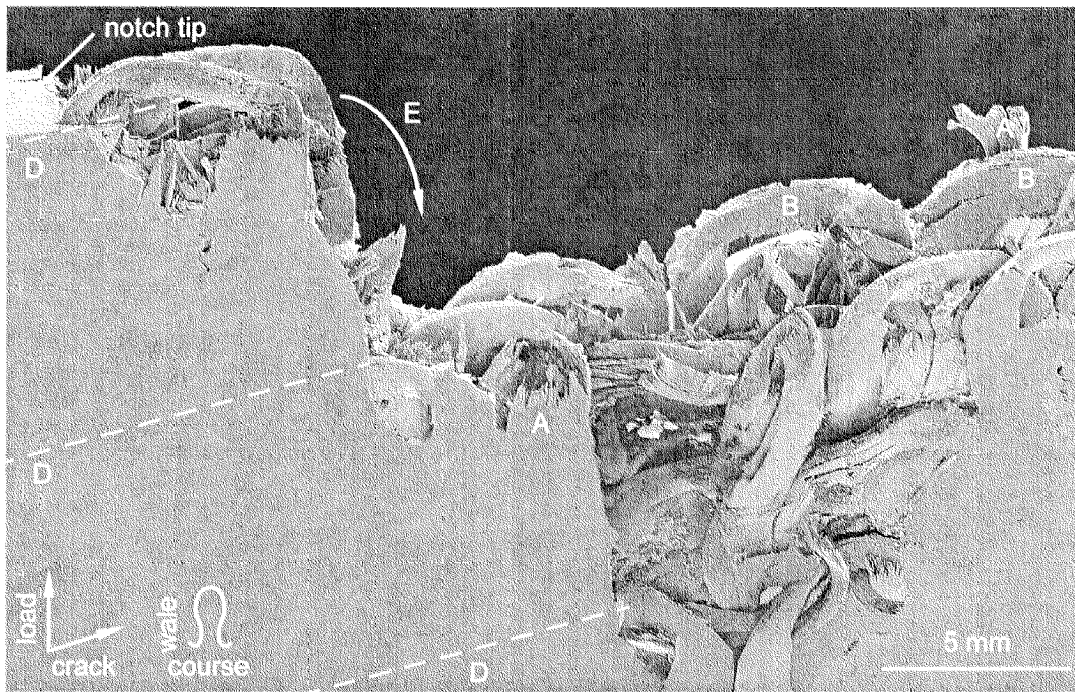
Figure 4.22: Overview of a fracture path resulting from compact tension applying load in wale. Because of bridging (E), the fracture path involves several loop rows (D). Side limbs (A) pinned the crack and failed in tension. Loop heads (B), oriented parallel to the fracture path, guided the crack.
