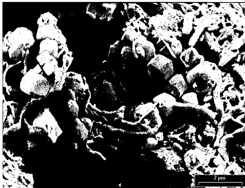
Figure 2.3: A scanning electron microscope (SEM) picture of the sewer biofilm from the village Rümlang showing the entrapped sand and zeolite particles (photo by I. Weidmann, EAWAG).
