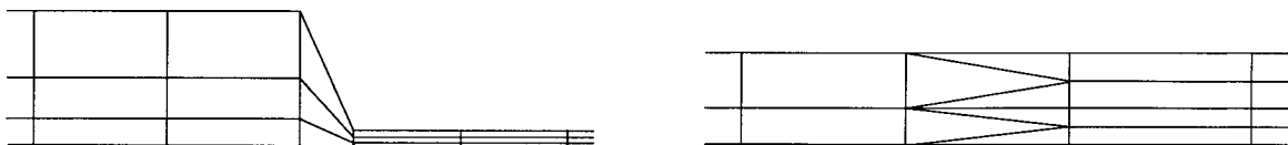
Figure 3.6: Left: bad quality elements are generated in the transition where the normal offsetting thickness jumps drastically; right: a better quality can be achieved by subdividing quadrilaterals
