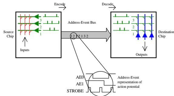
Address-Events are routed between chips under complete software control, thus preserving the reconfigurability of the neural networks implemented on the SCX system, a reconfigurability that is often absent in other, more specialised neural network hardware.
