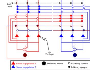
NB. Our technology allows us omit interneurons between 'inhibitory' neurons and excitatory synapses and *vice versa*, and in this example we have chosen to omit them, thus appearing to violate Dale's principal. However, we could equally well choose to accord with this principal by inserting the necessary interneurons.
