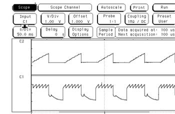
The lower trace (C1) shows the 'membrane potential' of one of the 'excitatory' neurons over time, and the upper trace (C2) that of the associated 'inhibitory' neuron.
