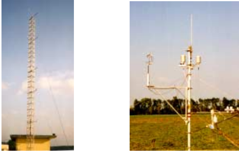
Figure 4.2.4: Left panel: 27-meter tower with 5 levels of additional meteorological measurements. Right panel: Small instrument tower A with eddy-correlation and additional instruments (see Siegrist, 2001).
