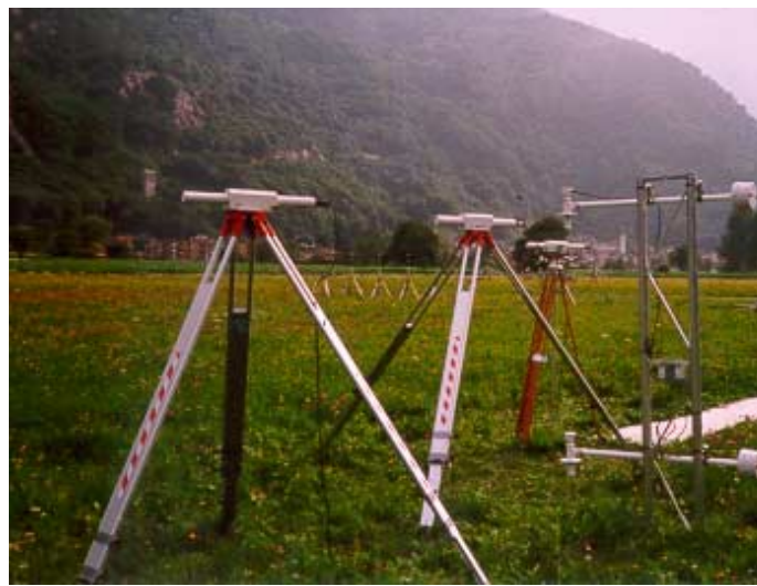
Figure 4.3.2: Set-up of displaced-beam scintillometers during the experiment in San Vitore. Path length of all scintillometers were R = 60 m. Additional temperature measurements were made with a small instrument tower, equipped with Pt-1000 temperature sensors (right side of the picture).
