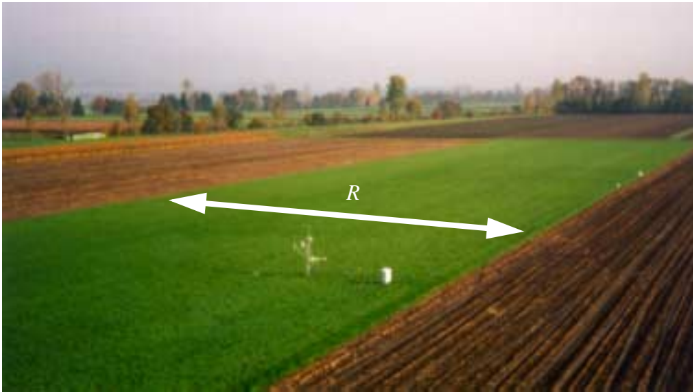
Figure 4.2.2: Picture of the measurement site near Kerzers, taken in November, 1998. The optical path R over homogeneous terrain is indicated by the arrow.
