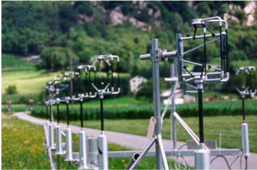
Figure 4.3.3: Array of sonic-anemometer-thermometers set up nearly parallel to the scintillometer paths.
