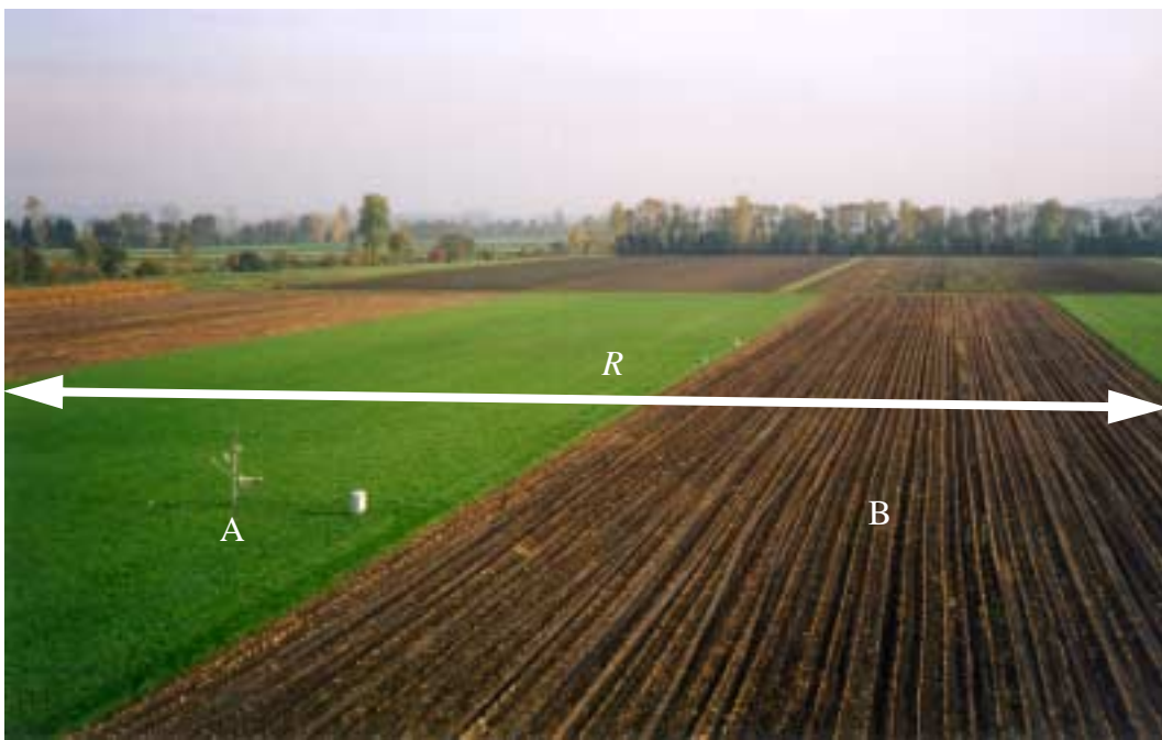
Figure 4.2.5: Picture of measurement site near Kerzers, with schematical depict of the optical path R over changing terrain. A and B mark the locations of the two small instrument towers A and B.
