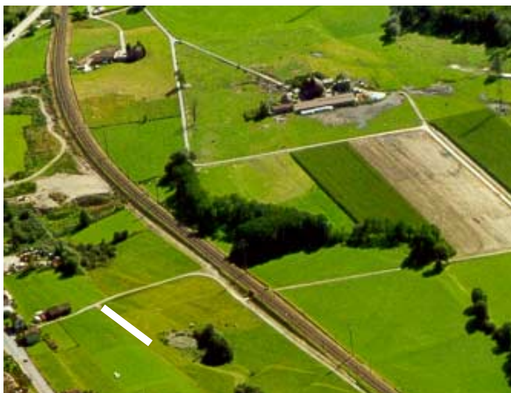
Figure 4.4.3: Picture of measurement site Torraza D , with schematical representation of scintillometer propagation path (white line). The site has a slope of 5.5^\circ perpendicular to the scintillometer path.
