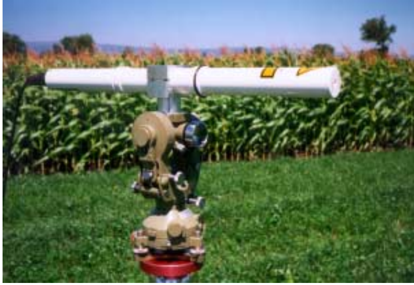
Figure 3.2.2: Emitter of the displaced-beam scintillometer, fixed on a theodolite for easier alignment.
