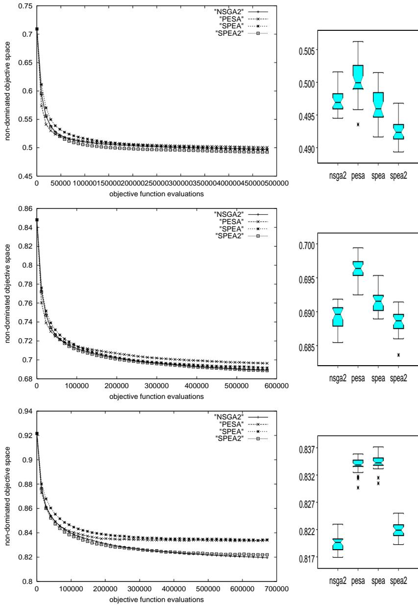
Figure 5: Performance values for KP-750- $m$  with  $m = 2$  (top),  $m = 3$  (middle) and  $m = 4$  (bottom). The graphs show the average values of 30 runs for each algorithm over time (left) and the box-plots of the distribution of all 30 samples at the end of the run (right).
