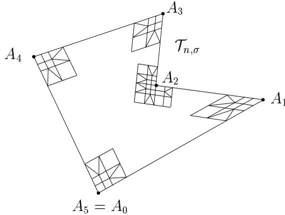
Figure 2: A geometric mesh  $\mathcal{T}_{n,\sigma}$  on  $\Omega$ .
