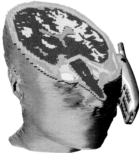
Figure 8.18: T250 phone model placed beside the high-resolution european female head phantom (HR-EF-1).
