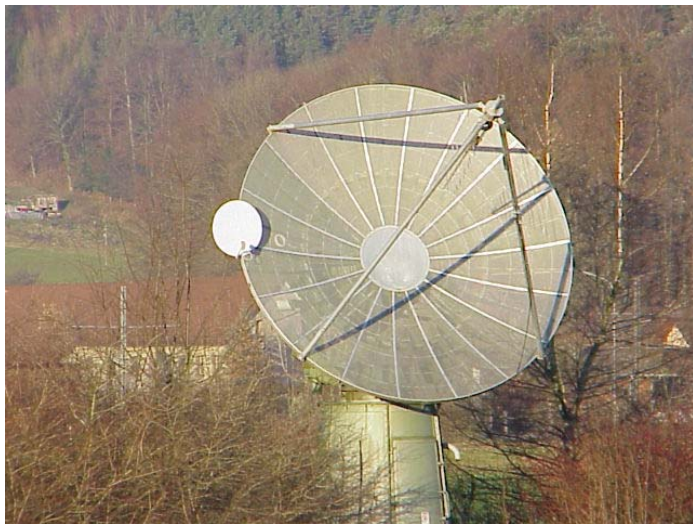
Fig. 1: 80cm satellite antenna mounted on a 5m dish antenna at Bleien observatory. The observatory with receiver and computers is 50m to the right side of the tower.
