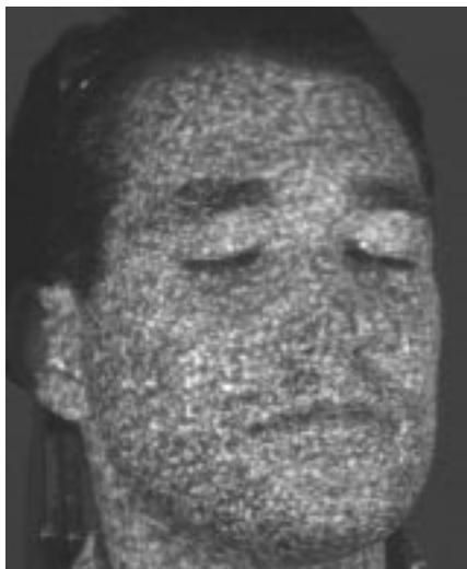
Fig. 4: Face with random pattern projection
