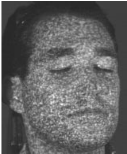
Fig. 4: Face with random pattern projection
