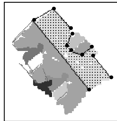
Fig. 9: Points for surface calculation projected to images space (endpoints of edges and DSM points)
