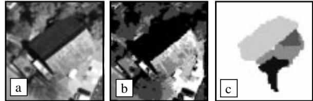
Fig. 13: Classification failure caused by radiometric properties: a) L\*-channel, b) classification result c) main roof surfaces
