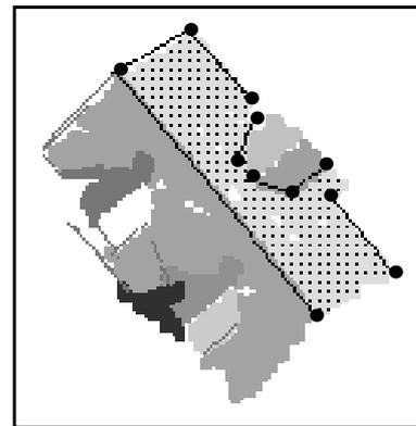
Fig. 9: Points for surface calculation projected to images space (endpoints of edges and DSM points)
