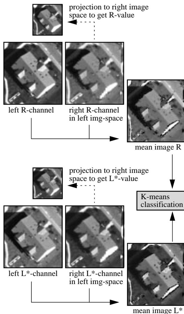
Fig. 6: Schematic view of the classification procedure
