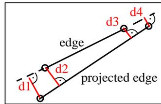
Calculation of a 3-D surface equation using one edge (start and endpoint and the projection centre) and projection of its corresponding edge in the other image onto this surface leads to a 3-D edge (Fig. 8).
