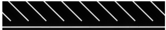
Figure 13. Self-made test patterns used for correction of vibrations and partial image scanning errors (displayed image has been rotated by 90 degrees).
