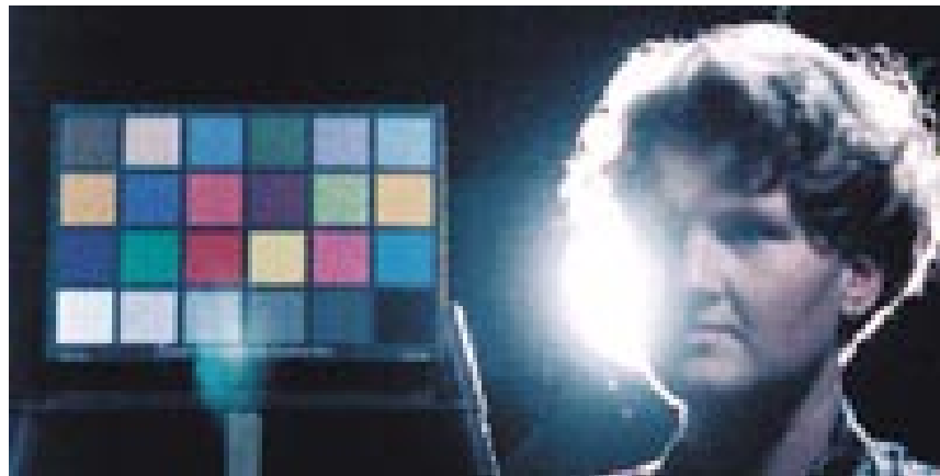
Left: High Dynamic Range CMOS camera (logarithmic response, dynamic range beyond 140 dB) Right: standard CCD
