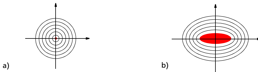
Figure 7.14 Isolines of a) a spherical, symmetric primitive and b) a new ellipsoidal primitive.
