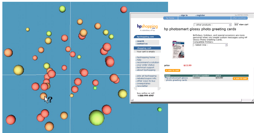
Figure 9.7 Snapshot of a VisMine scene showing a set of clustered product objects. Additionally, detailed info is shown in an extra for a product of special interest. [HP©].
