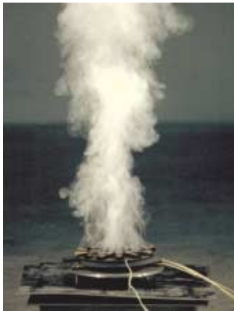
Figure 8. One of the prescribed testfires: smoldering combustion of beech wood. When the fire stopped, the NO 2 -concentration was 140 ppb.
