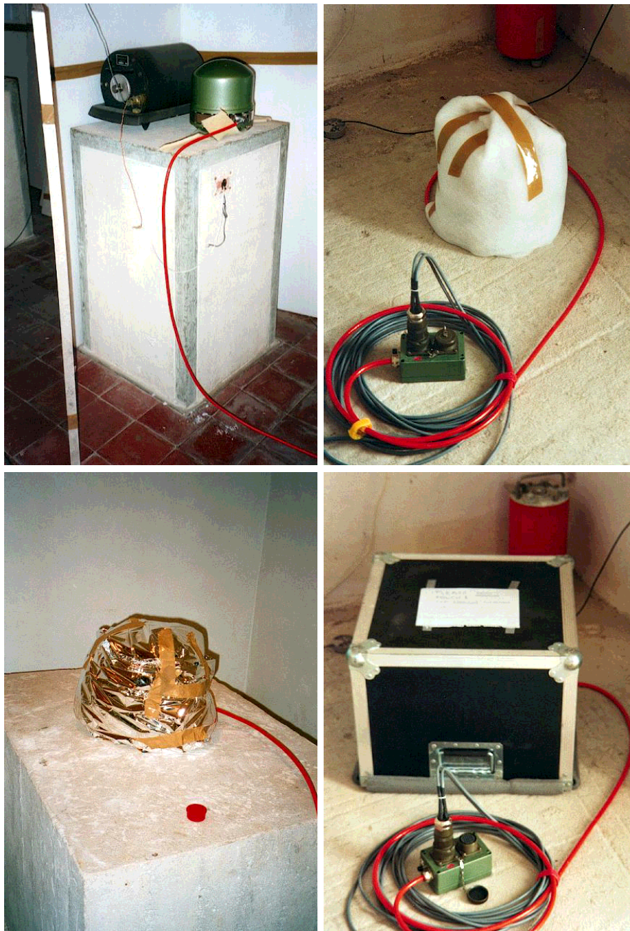
Figure 2.3: Installation procedure: STS2 seismometer (top left), wrapped with cotton wool (top right) and a radiation reflecting rescue sheet (bottom left), everything covered with a styrofoam box (bottom right).
