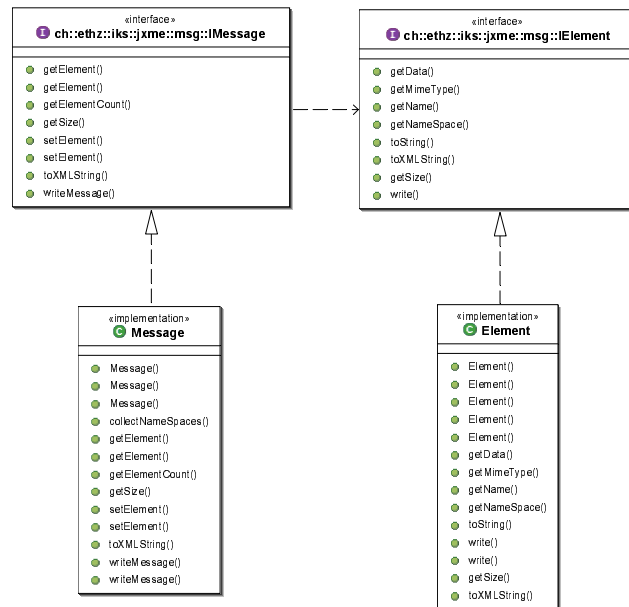
Figure 3.4: UML Diagram of a Message and its Elements
