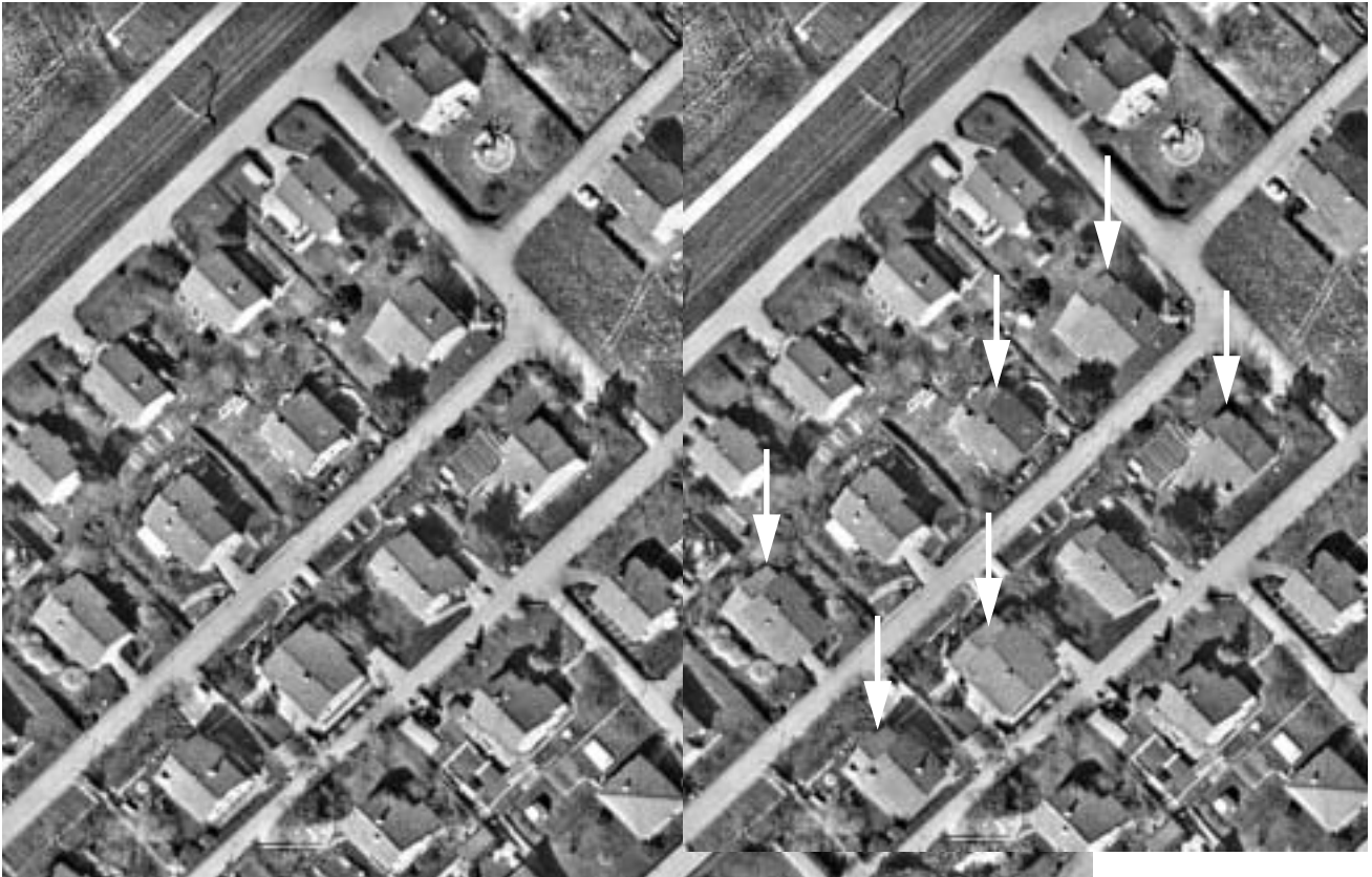
Figure 1. Ortho-image: (left) houses are radially displaced, (right) the houses indicated by the arrows are corrected a posteriori.
