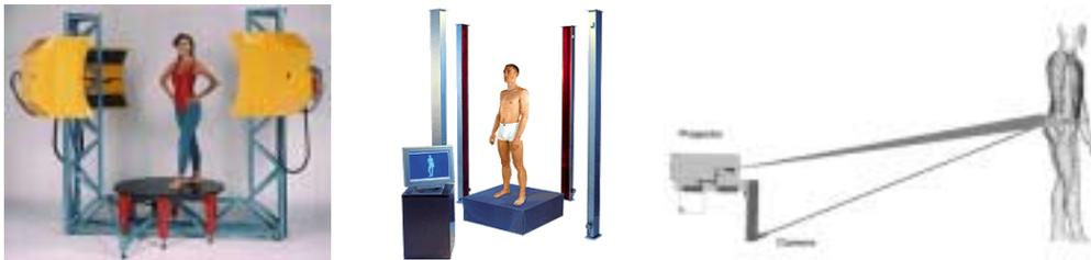
Figure 1: Two examples of 3D body scanner: Cyberware [8] (left) and Vitronics Vitus [25] (center). The triangulation process between projector camera and target subject.
