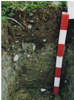
Fig. 4.8 Soil profile P 23 in Ror catchment. Grey colour and rusty mottles indicate frequent saturation of subsoil.
