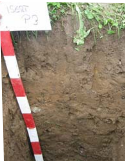
Profile excavated down to 85 cm, drilling possible down to 195 cm.
