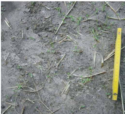
Fig. 4.7 Surface crust formed by soil surface sealing in Isert catchment.
