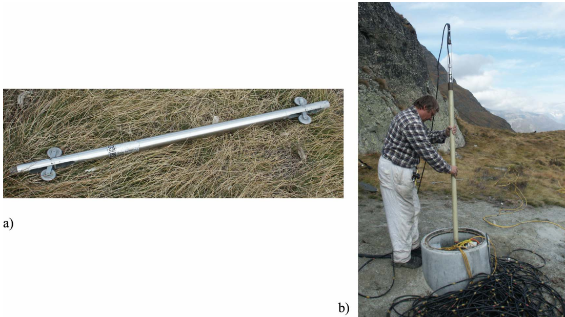
Figure 3-15: a) Photograph of the inclinometer probe which is 61 cm long. b) Photograph of the 2 m long INCRES extensometer probe being lowered into a casing. (Photographs by E. Eberhardt)
