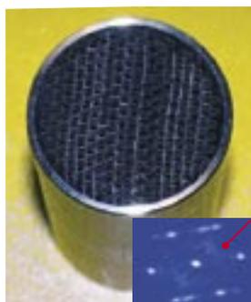
X-ray picture of catalytically active platinum particles.
