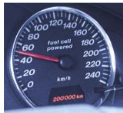
**Long-lasting:** Fuel cell membranes have achieved a service life corresponding to 200,000 km at an average speed of 50 km/h.
