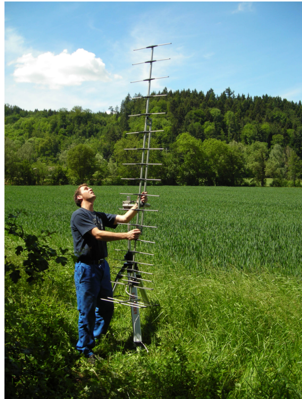
Fig. 1. Eastern side broadband TV-antenna of the solar interferometer at Bleien observatory. H. Meyer is carefully adjusting the antenna on a tripod to be pointed to Cygnus A.
