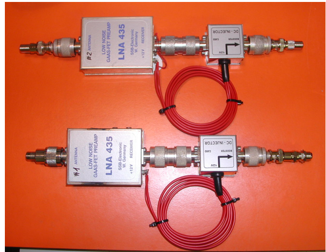
Fig. 3. Two GaAs-FET low noise preamplifiers tuned to 458.71MHz. Each preamplifier was combined via a Bias-T to F-type cable adapters. According to their specifications, these LNA's have a noise figure NF in the order of 0.7dB (52Kelvin).
