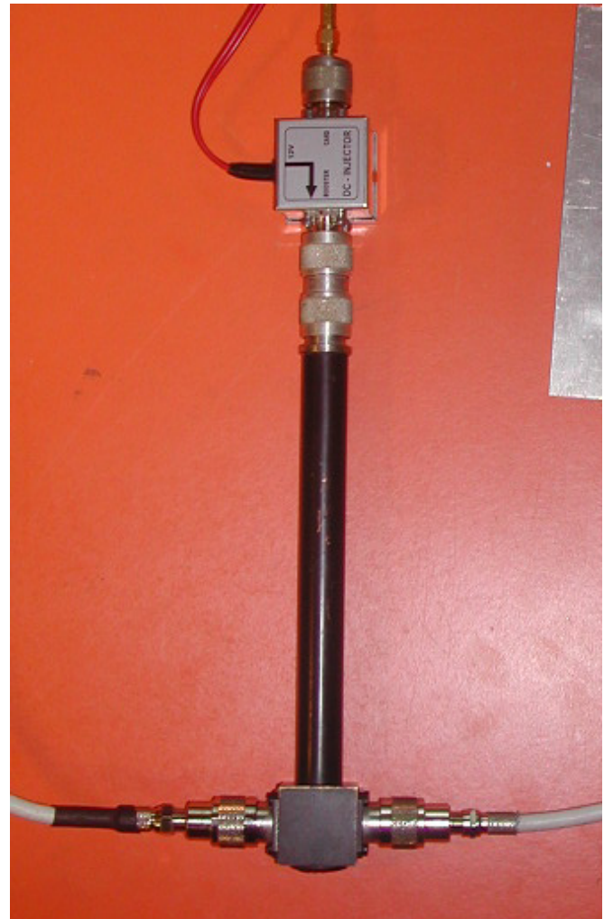
Fig. 4. On top of the combiner a Bias-T was connected to a power supply to energize the preamplifiers with 12V dc. Eastern element cable (bottom left) and Western element cable (bottom right) were fed to a quarter wave power combiner.
