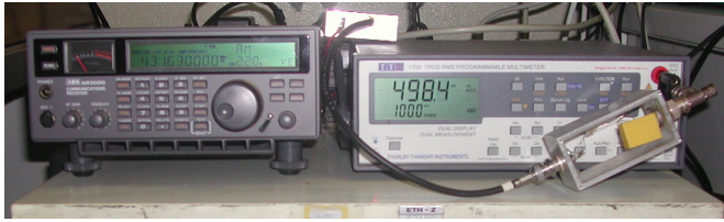
Fig. 5. The radiometer (left) is a commercial communication receiver AR5000 fully programmable via a serial line from a PC. The digital multimeter (right) samples the analog voltage taken from the logarithmic detector AD8307 (middle top) and stores the data on a PC. In front of the multimeter we see a passive integrator (first order low pass filter) composed of a 1 Megohm resistor and a 1 microfarad capacitor.
