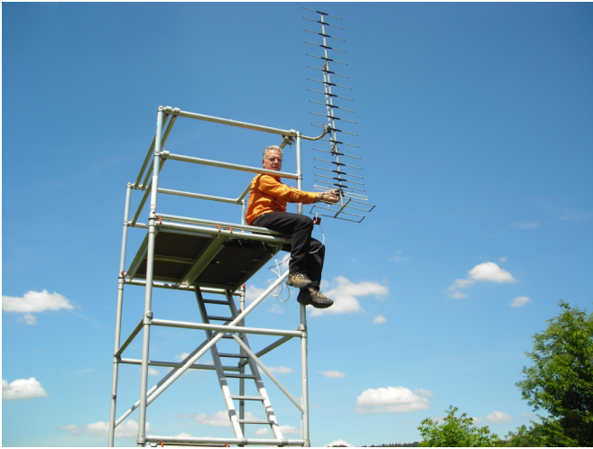
Fig. 2. Western side broadband TV-antenna of the solar interferometer at Bleien observatory. The other author, on top of the scaffold is checking the cable connection at the dipole.
