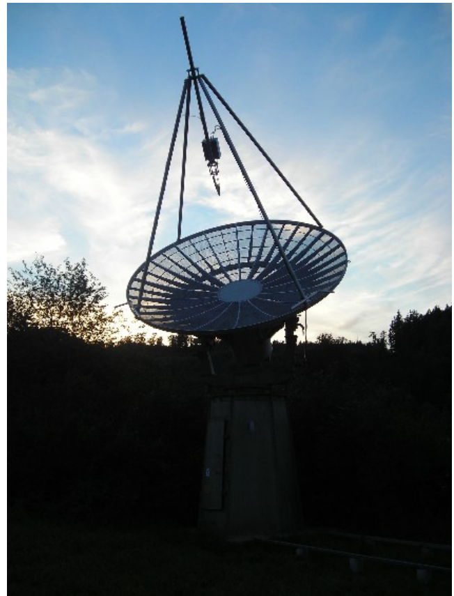
Fig. 1. 5m radio telescope in twilight at Bleien observatory. A logarithmic periodic dipole array is mounted in front of the FPU.
