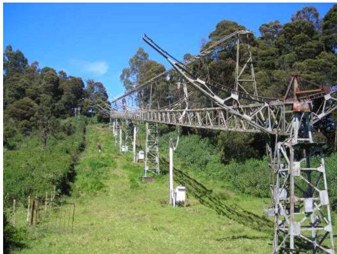
Fig. 1. Dipole array Muthorai 500m x 30m at 327MHz dedicated to solar radio observations.
