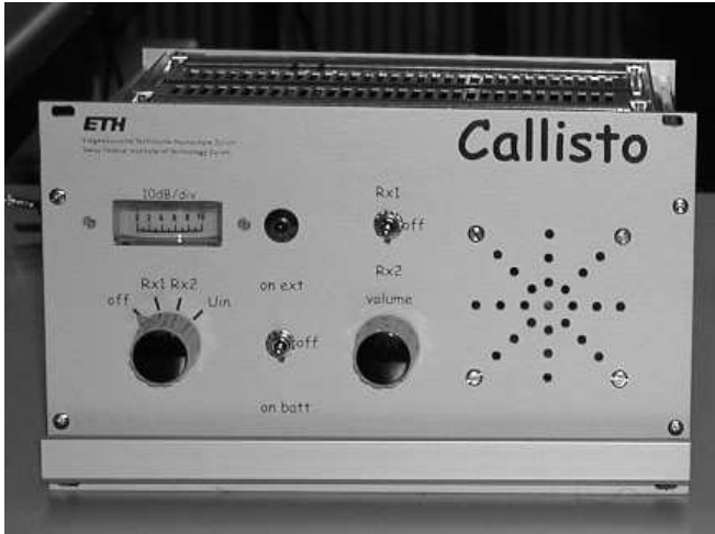
Fig. 2. CALLISTO dual receiver, frequency agile spectrometer foreseen to upgrade Ooty for solar spectroscopy.
