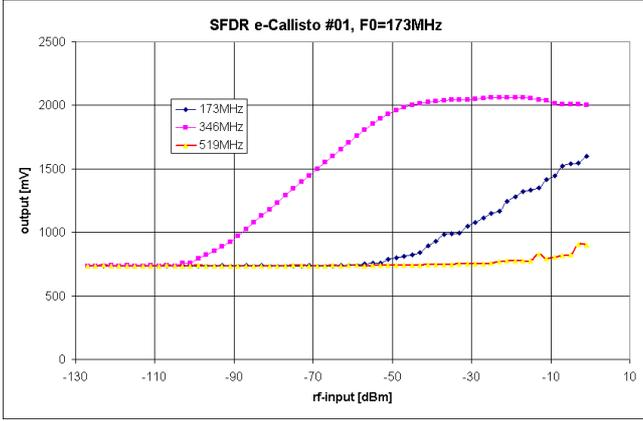
**Fig. 6.** Spurious free dynamic range at a standard gain voltage of 2.0Volts. SFDR is clearly above 40dB.
