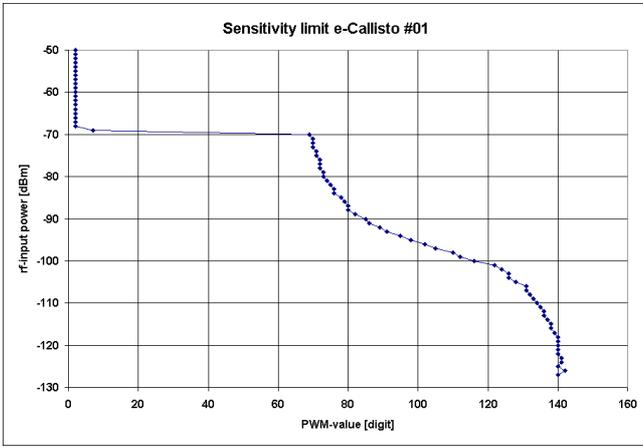
**Fig. 7.** Sensitivity limit as a function of applied pwm -value to the PWM-port of the RISC system.
