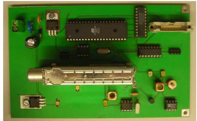
**Fig. 1.** Electronic board of double super-heterodyne spectrometer e-Callisto including tuner and RISC processor.
