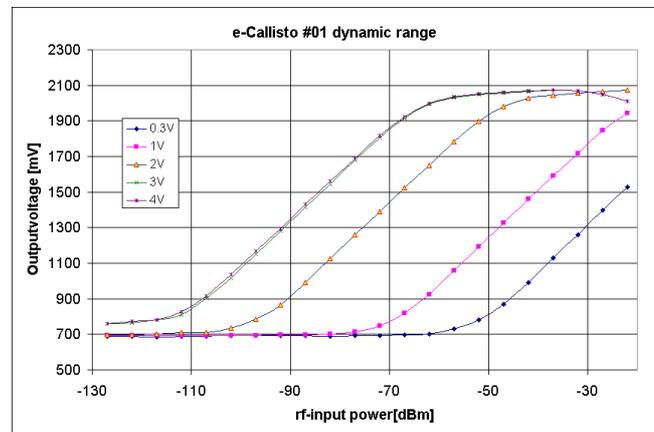
**Fig. 5.** Dynamic ranges as a function of gain voltage.
