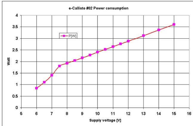
**Fig. 3.** Power consumption as a function of applied input voltage. E-Callisto supply range is limited between 8V and 15V dc. Nominal supply is defined to 12Vdc.
