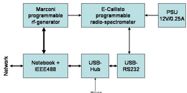
**Fig. 2.** Schematic of the automated test system using IEEE488 bus concept.
