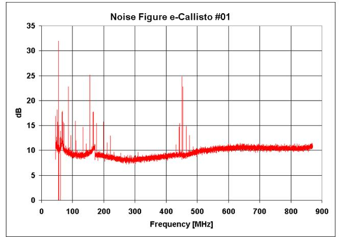
**Fig. 9.** Noise figure of e-Callisto (without preamplifier) using hot-cold-method. NF in average is below 10dB.
