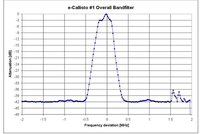
**Fig. 8.** Overall band filter response at 150MHz.
