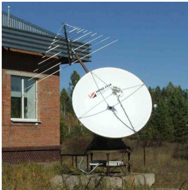
Fig. 1. Linear polarized, logarithmic periodic dipole mounted at one of the interferometer dishes in Badary. The dish in front of the observatory automatically tracks the sun day by day.
