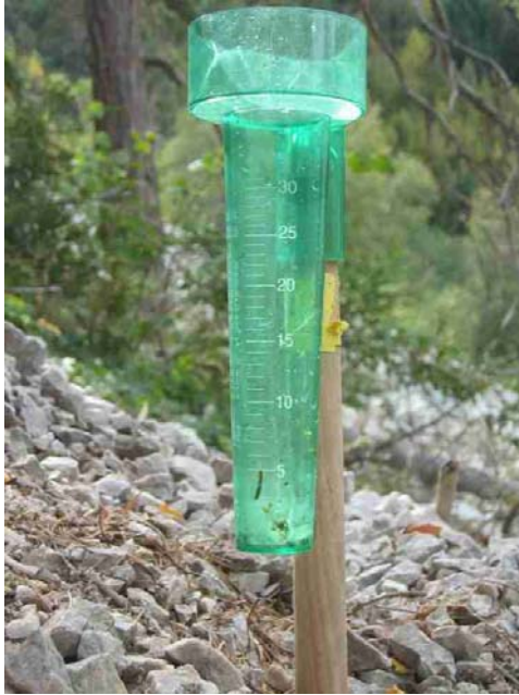
Figure 4-26 Rain gauge for the measurement of the plot site precipitation
