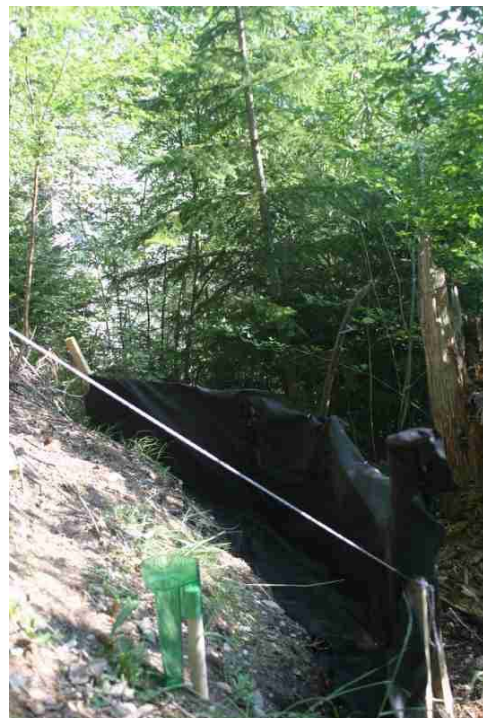
Figure 4-15 Silt fence plot C2 (Corina Gwerder)
