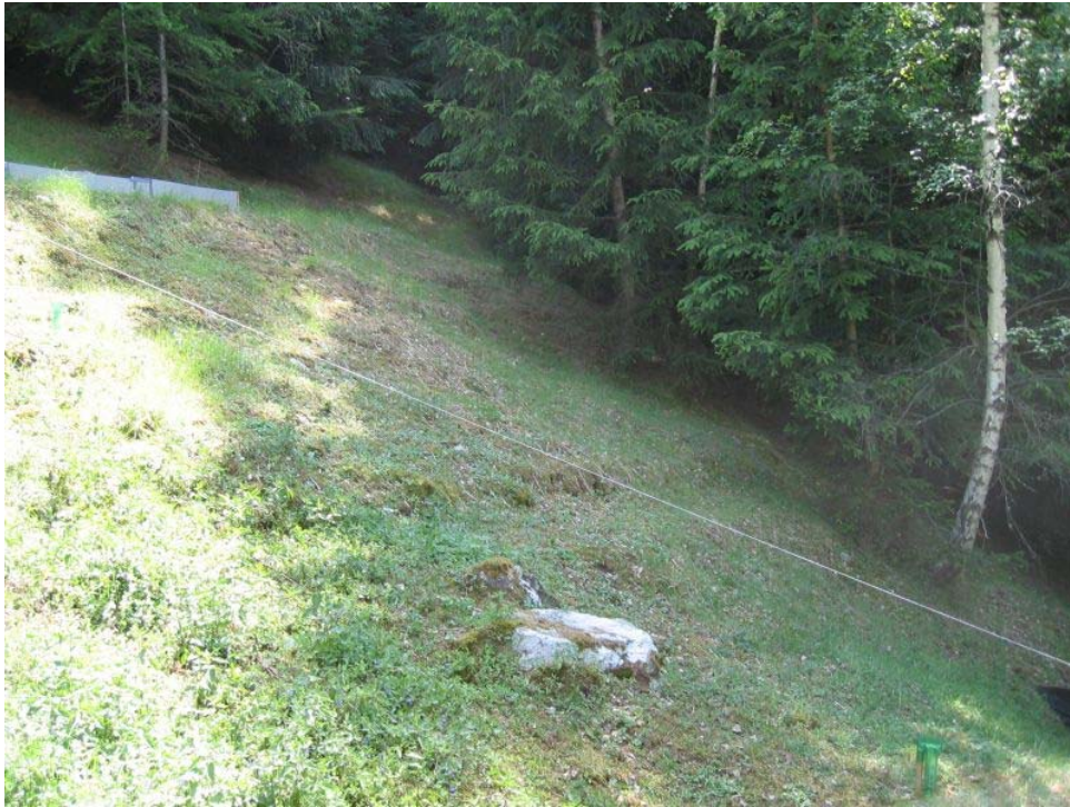
Figure 4-10 Silt fence plot B2, the pvc plate forms the upper barrier (Corina Gwerder)
