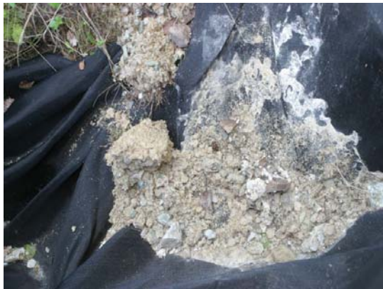
Figure 4-33 Silt fence sediment content example at plot A2 (Corina Gwerder)
