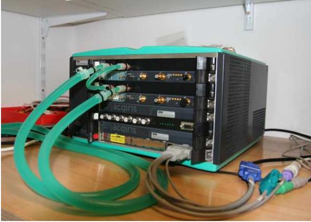
Fig. 2. Eight slot crate sold by Acqiris company, Geneva. The crate holds two AC240 sampler cards, an I/O interface card and a slot PC.
