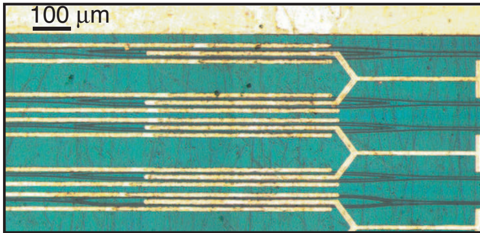
Figure C.4: Mach-Zehnder modulators. The ridge waveguides have width from 3 to 10 \mu\text{m} .
