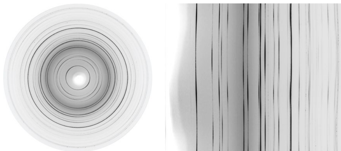
Figure 3.4: Synchrotron diffraction data of a PS/Offretite sample prepared by the modified matrix-smear method (left), unrolled pattern 2\theta vs. azimuth 0-360^\circ (right)
