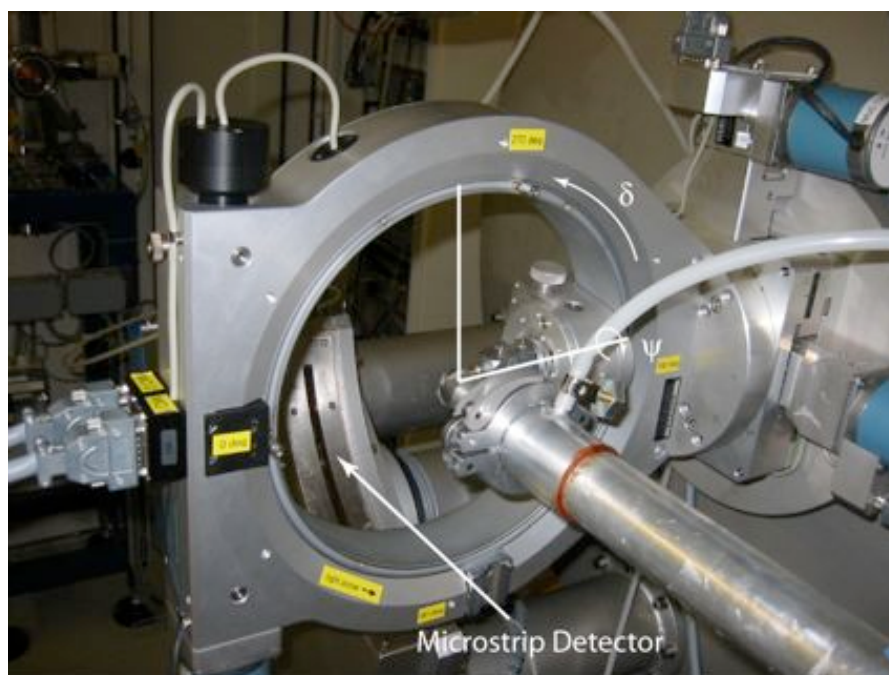
Figure 4.3: The setup on the Material Science beamline at the SLS, showing the beam pipe, the Eulerian cradle with the rotation axis \psi and the tilt angle \delta and, indicated at the back, the entry slit to the microstrip detector
