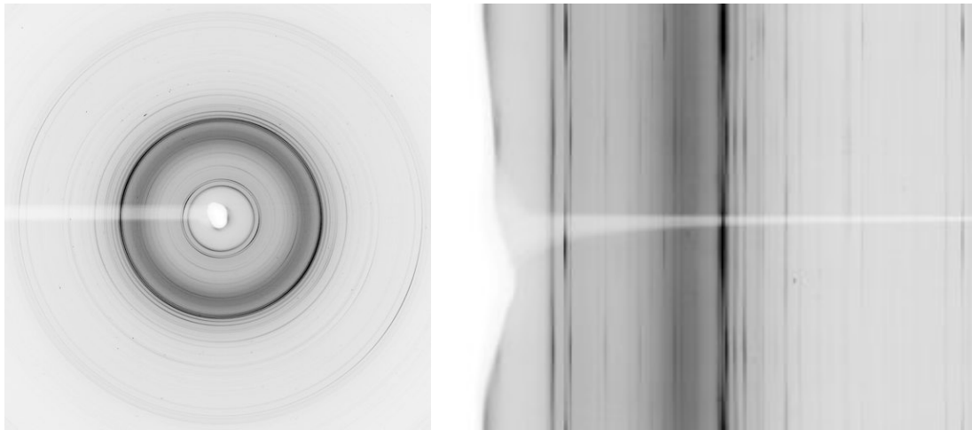
Figure 3.8: Data from a PS/IM-5 sample prepared using the repetitive pressure molding collected using the 2-dimensional PILATUS 6M detector on the X06SA PX beamline at the SLS (left), and the unrolled pattern 2\theta vs. azimuth 0-360°. Note the intensity variations corresponding to different sample orientations indicating that preferred orientation had been induced.
