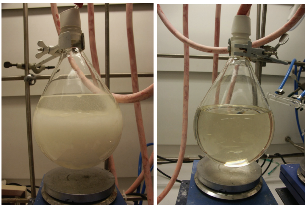
Picture 22: Clarification of mixture upon addition of pTSA. It is important that the solution becomes clear. Undissolved material or turbidity indicates that the quality of the dihydroxyacetone dimer used is not good and problems might result in the following step.
