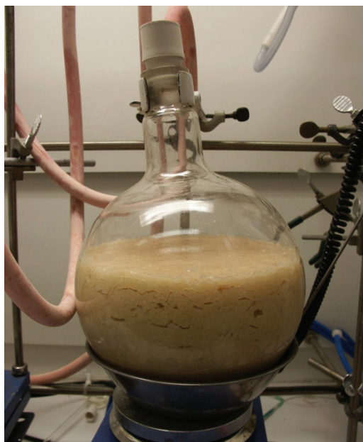
Picture 27: The mixture adopts the consistence of mud and should be shaken with ether remove it from the flask.
