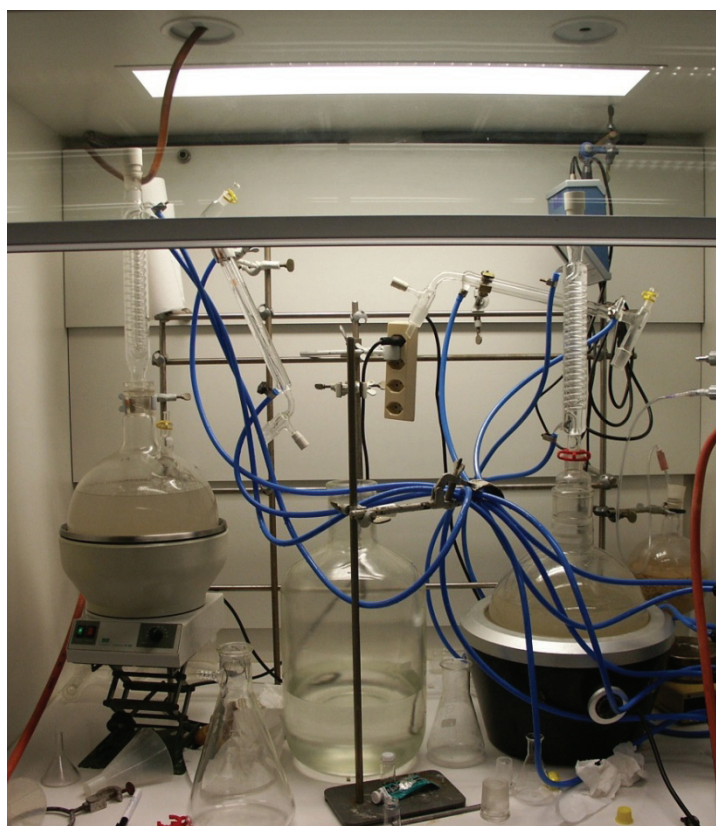
Picture 28: Two apparati for the refluxing step. Bumping will occur, but is usually no problem for the reaction.
