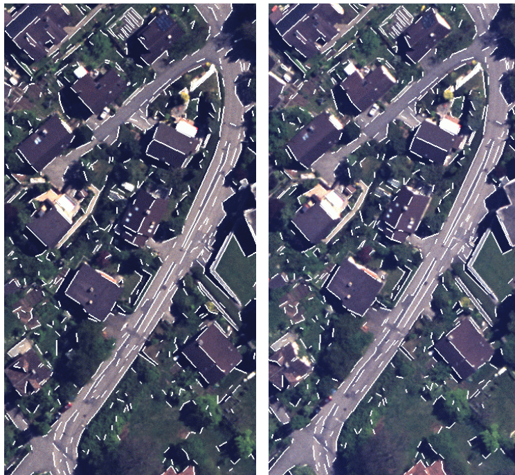
Figure 7. Result of straight line matching in a stereopair
