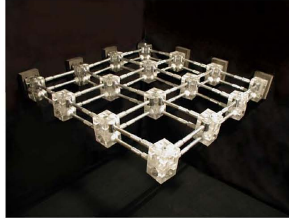
(b) SmartMesh prototype reproducing a plane
