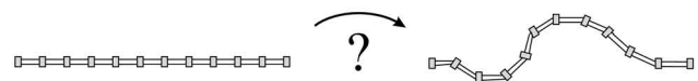
Figure 3: Finding an actuation plan in order to deform the SmartMesh from an initial state to the desired final one.
