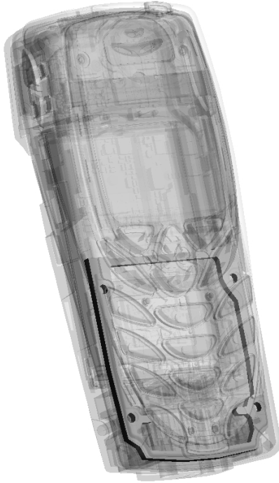
Figure 6.11: SEMCAD X model of the Nokia 8310. The support frame (highlighted) was coated using a conductive spray, which then acts as a grounding mechanism between main and keypad PCBs. Integrated into enhanced FDTD platforms [66] the novel algorithm allows the simulation of such complex 3D real-world problems including EMI and metallic coatings which could not be performed by the standard Yee scheme.
