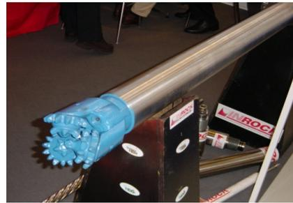
Figure 2. Mud Motor with roller bit.
