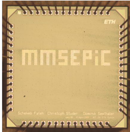
Figure 3.10: ASIC micrograph of the SISO MMSE PIC detector in 90 nm (1P/9M) CMOS technology.
