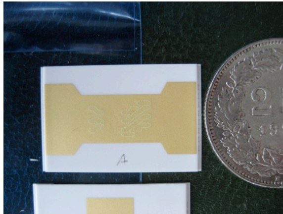
Figure 7-10 Realized Butler matrix in LTCC at 60GHz
