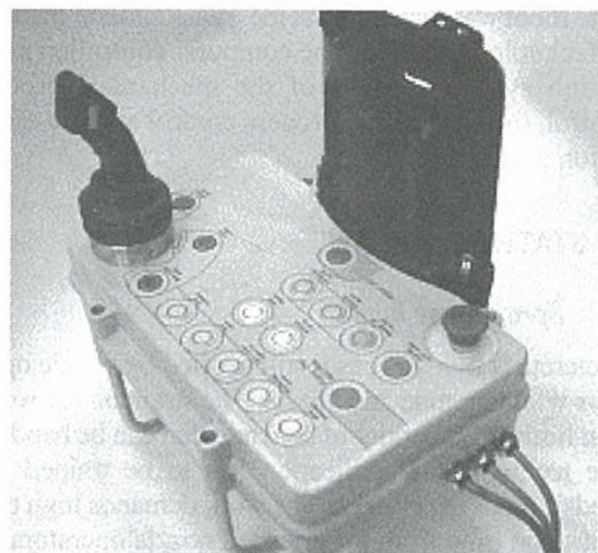
Figure 3. Remote control with 6D-joystick.
