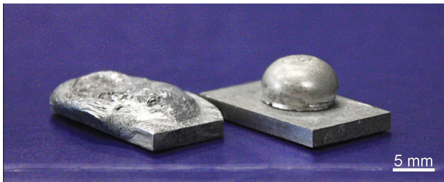
Fig. 3.5: Poor wettability of the untreated AZ31 substrate with oxide layer (right); excellent wettability of the Zn-coated and heat-treated substrate (left).
