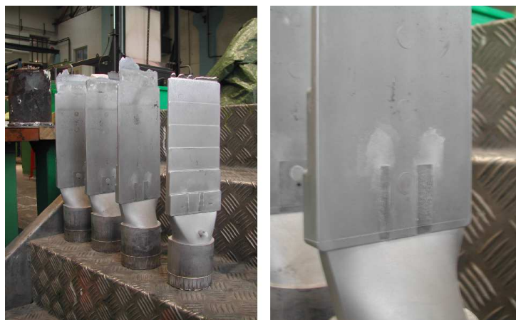
Fig. 4.9: The compound cast component with an insert featuring various thicknesses. The Zn coating partially shears off when liquefied by the melt.
