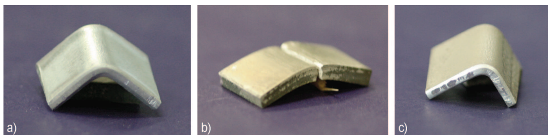
Fig. 2.21, a - c: Coated samples after bending. Zinc on aluminium (a), zinc on magnesium (b) and manganese on aluminium (c). None of these coatings start to peel off the substrate.
