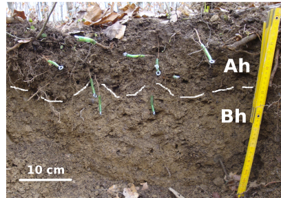
Figure 4.3: Field soil profile showing roots of spruce ( Picea abies ) with metal rings ready for a pullout experiment.
