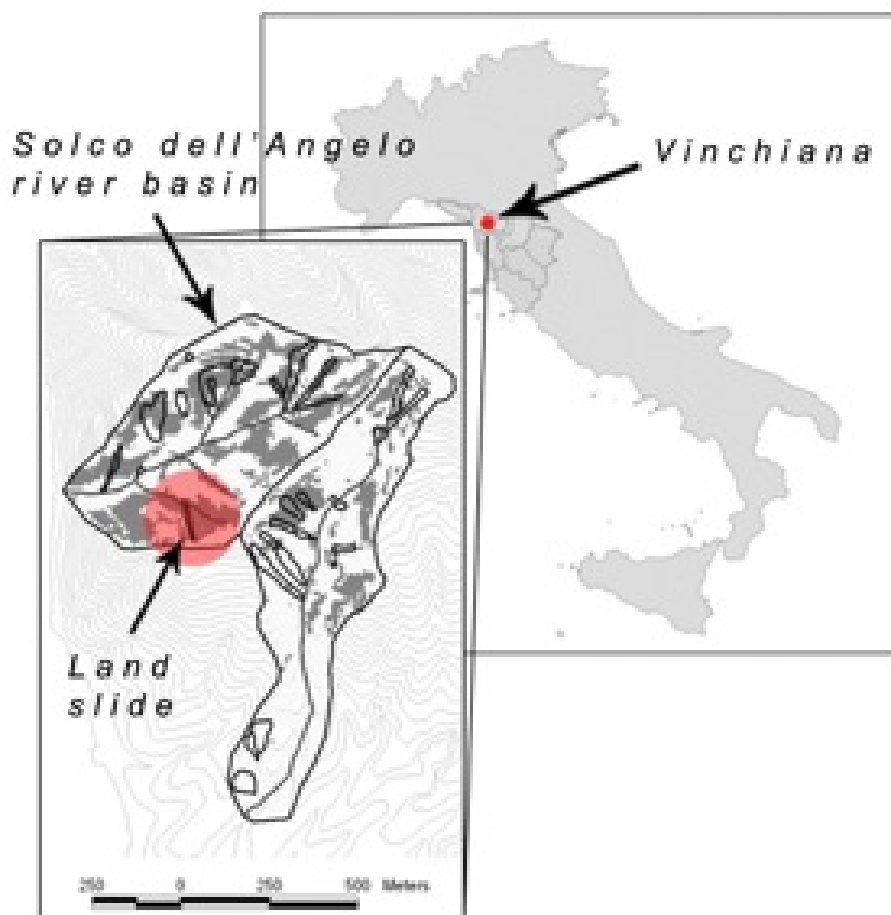
Figure 6.1: Localization of the Vinchiana (Tuscany, Italy) case study and landslides map: black-lines landslide contours and in dark colour areas with SF 1 estimated by the infinite slope model during the November 2000 event and in (Solco dell'Angelo and Piantone basin).
