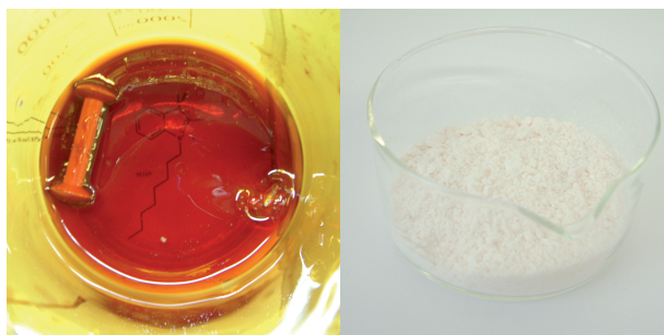
Figure 4.4: The red transparent 28 as iodide in a beaker with the molecular structure on paper underneath (left hand side) and the isolated and dried white crystals of 28 as perchlorate (right hand side).
