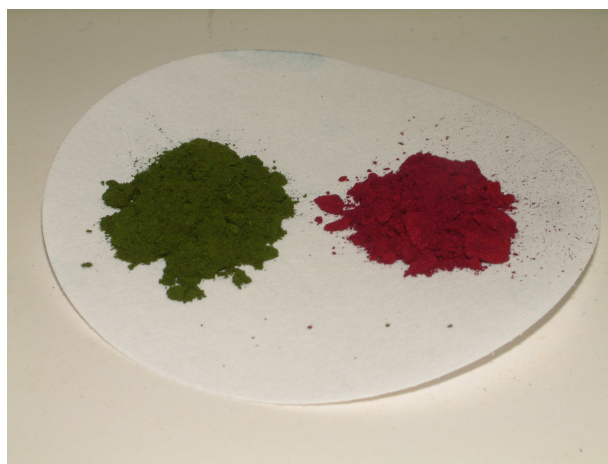
Figure 4.2: Picture of the solvent-free, golden-green crystals (left hand side) and the copper-red chloroform adduct of 12 .
