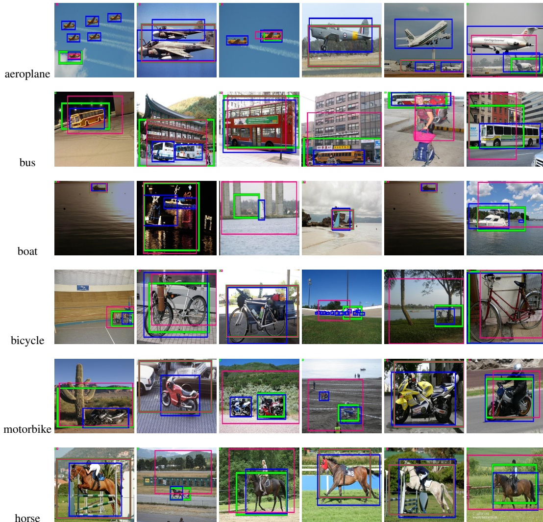
Figure 3.3: Localization results for Divide and conquer LocLearn. Blue windows represent ground-truth, pink windows are the ones selected by LocLearn setup (d) in Table 2.1 and with green are colored the final windows selected in the localization stage by Divide and Conquer LocLearn setup (g). There are images for which the 2 algorithms return the same labels, but on average the green windows are better as the results in Table 3.5 show.
